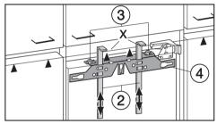
■ Undo nuts ③ and take fixing bracket ④ off together with fitting aids ②.
